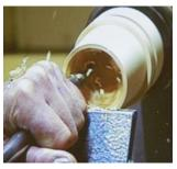
The part that was to be the lid was then mounted in the chuck and with an engineering drill in the tailstock, Mike drilled out the centre, using a slow speed and withdrawing the drill regularly to keep the bit clear of shavings.
