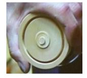
He then hollowed out the base and used a home-made scraper (made from an old planer blade) to clean up the inside. Mike then removed the base from the chuck having first made a pencil mark on the base to align with a "nick" that he has filed on one jaw of his chuck. This enables the piece to be returned to the chuck aligned exactly as before.
